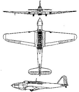
A Fairey Battle, low-winged monoplane, used by the RAAF for bombing and gunnery training at Evans Head, New South Wales, and Port Pirie, South Australia. This aircraft had a maximum speed of 410 kph at an altitude of 4600 metres. In early 1942, Air Board estimated Australia's requirement for the plane to be 336 airframes and 448 engines (*Gillison, p.86*). It is interesting that pilots complained that the Fairey Battle was "too easy to fly".
