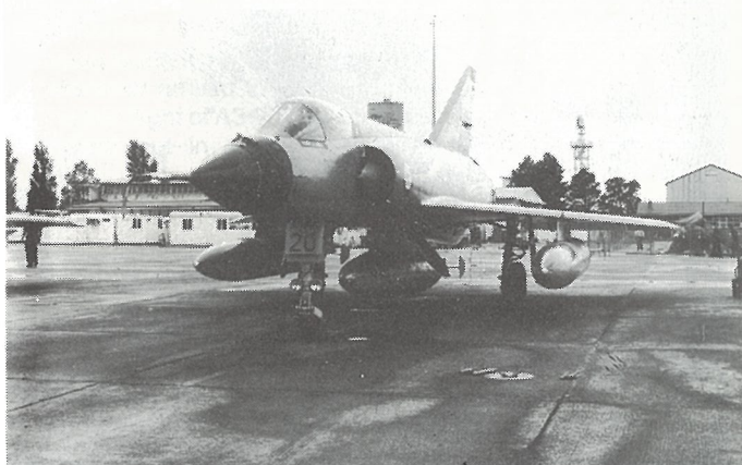
A3-20 with max external fuel configuration 24 January 1986. (RAAF)
