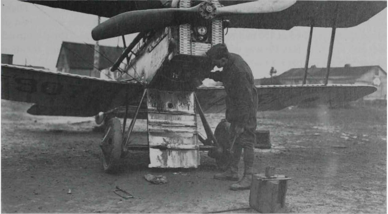
*An Australian mechanic with the lower engine cowl dropped to allow access to the SE-5A's Wolseley engine* AWM D439
