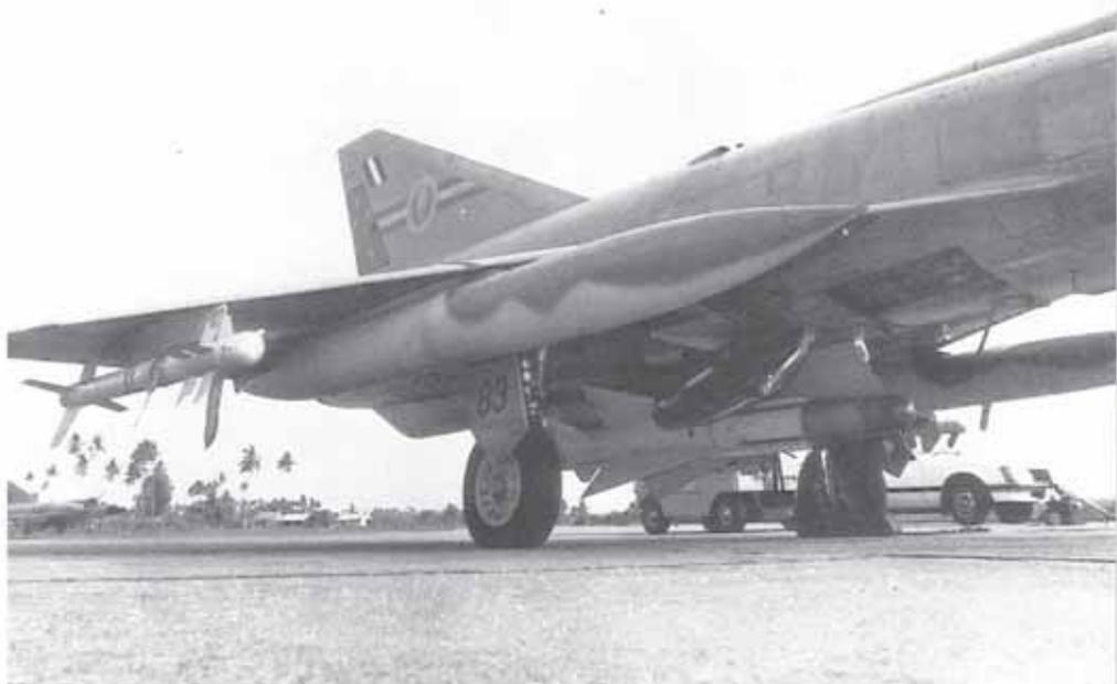
*First RAAF Mirage to be loaded with Matra "Magic" Missile. Standard Matra Missile fitted under centre fuselage.*
